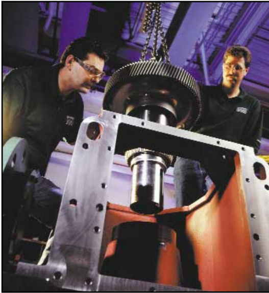
Reassembly of a 700 series reducer after repair.
