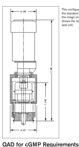
This configuration shows the standard single seal; the image on the front shows the optional double seal unit.
