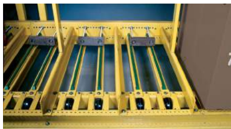
Battery compartment with adjustable back stop.
